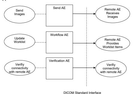
Figure 4-1 Ambu aBox 2 DATA FLOW DIAGRAM
