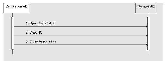
Figure 4-5 SEQUENCING OF ACTIVITY: VERIFY CONNECTIVITY WITH REMOTE AE
