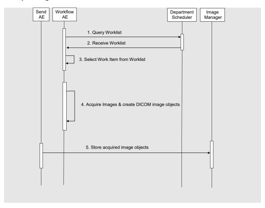
Figure 4-2 SEQUENCE DIAGRAM – IMAGE ACQUISITION AND ARCHIVING TRIGGERED BY WORKLIST
